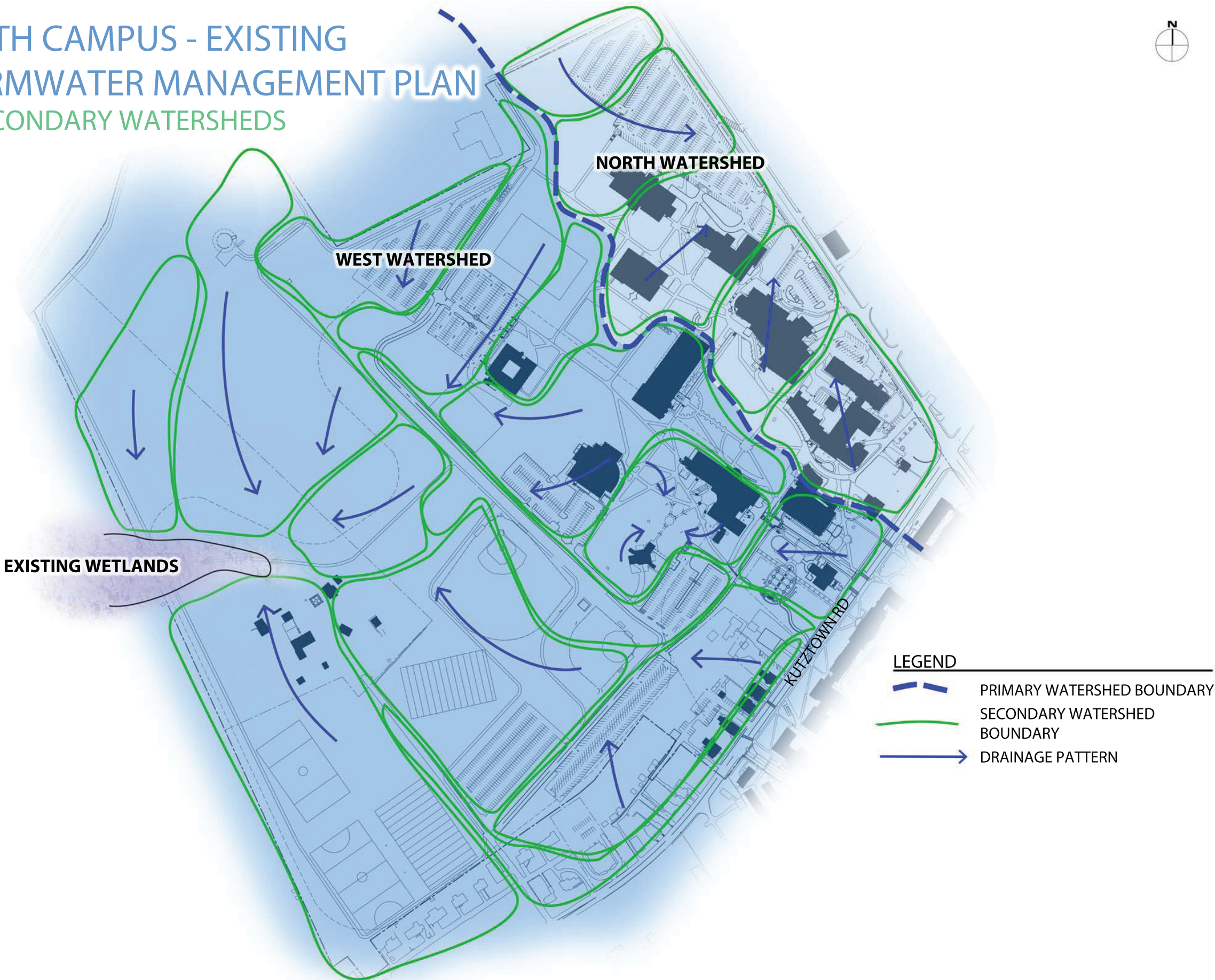
Diagram 3.13.2 - North Campus - Existing Stormwater Management Plan: Secondary Watersheds
