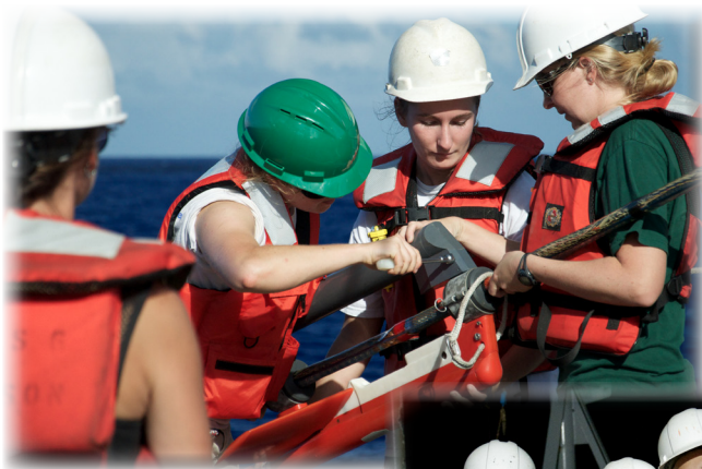
Above, Jen Herting and Dr. Oakley working on the fantail, installing a flotation device onto the seismic streamer during deployment with a crew member and seismic technician. At right, Tom Bond, Dr. Oakley and Nick Mathews pause for a picture.
